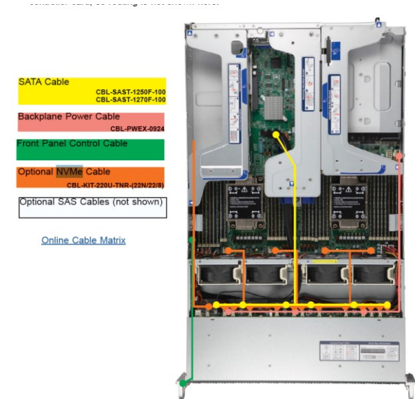
Figure 3-18. Cable Routing Diagram
